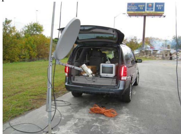
WA3CPO 3480MHz receive setup at the Harrisburg HACC training site. About 15 miles from the N3TWT repeater
